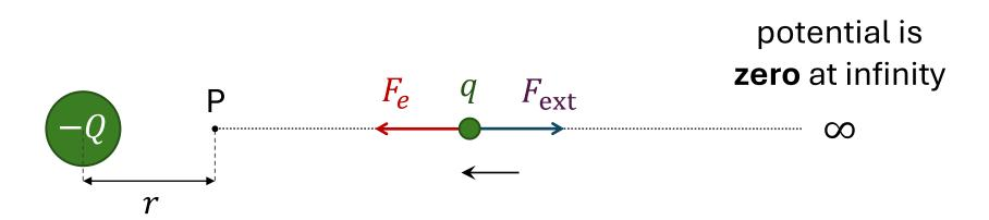
The electric potential at a point is defined as the work done per unit charge (1 C) in bringing a small positive test charge from infinity to that point.
